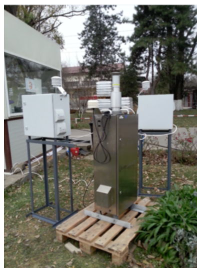
Fig.3. Inter-comparison tests for PM_{2.5} monitors calibration performed in Bucharest (left and right - two RokidAIR PM_{2.5} micro-stations; centre - a Leckel SEQ 47/50 Sequential Gravimetric Sampler provided by NILU).
